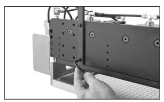
Figure 15. Installing the vertical fence.
